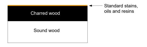
The CWT permeates the charred part deep down up to the sound wood. The homogeneity thus obtained associated with the adhesion capacities of the product guarantees a very good resistance to bad weather, infiltration and friction.
